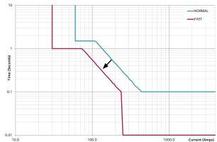
Fast curve i<sup>2</sup>t is a configurable fraction of the normal curve i<sup>2</sup>t
